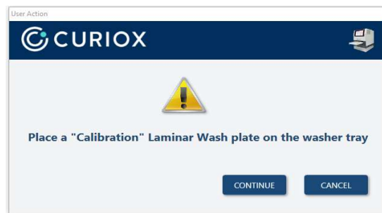
Figure 4-16. Prompt to remind User to place Calibration plate on washer tray following priming.
