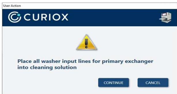
Figure 4-63. Prompt for Users to set up the primary Buffer Exchanger for Shutdown Maintenance.
