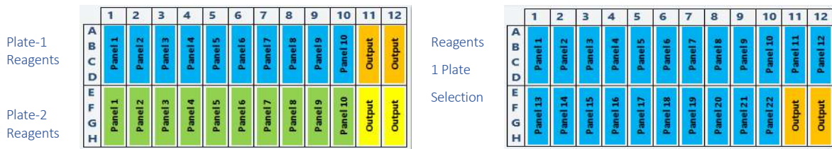
Figure 4-31. Reagent Plate layout for two sample input plate (left) accommodating 10 panels / reagents each, or reagent plate layout for one sample input plate (right), accommodating 22 panels / reagents in Total.
