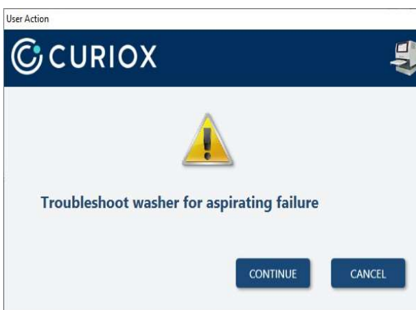
Figure 4-20. Prompt to perform troubleshooting if aspirating failure was reported on Step 5.
