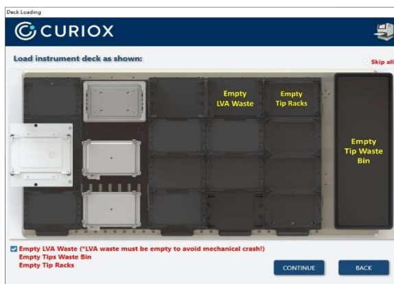
Figure 4-47. Guide to prepare deck for run – empty waste from Tip Waste bin and AUTO1000 deck spaces.
