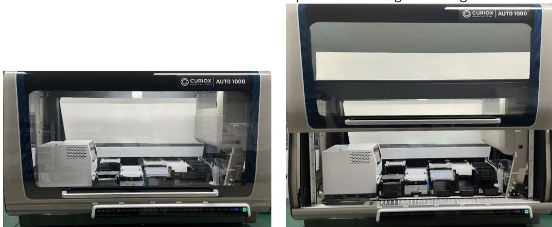
Fixture 2-4: (Left) User pulls handle to open door. (Right) Door is opened for cleaning or deck loading purposes.
