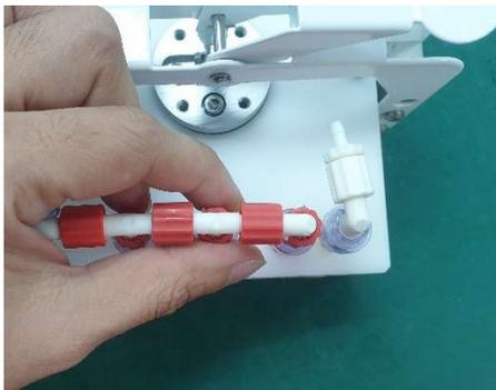
*Figure 5-3: Disconnecting the Inlet Joint*
