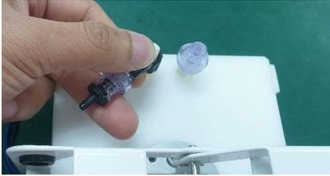
*Figure 5-6: Disconnect the Overflow Outlet*
