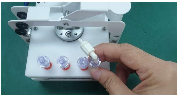
*Figure 5-5: Disconnect the Waste Outlet*
