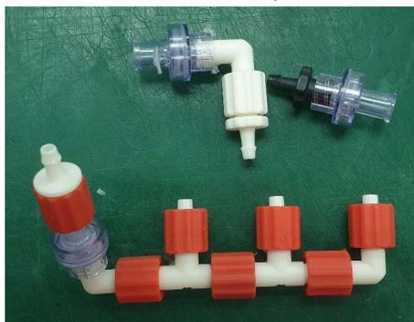
*Figure 5-10: Reassemble Connector Joints to Clamper*
