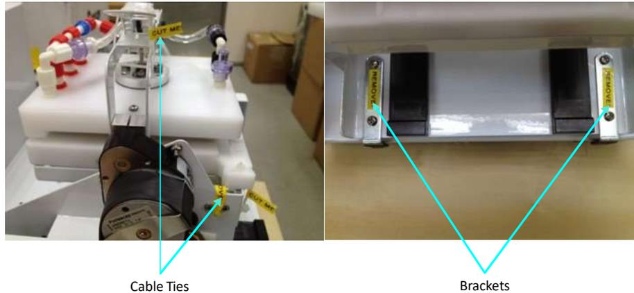
**Figure 3-2:** Cable ties and brackets to be removed before powering the LT-210MX on.
