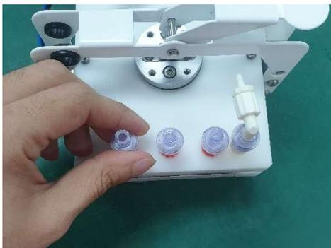
*Figure 5-4: Loosen the Check Valve*
