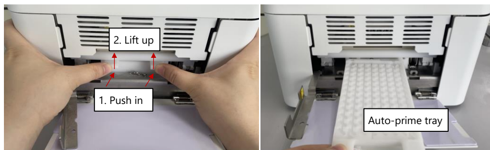
Figure 4.3: Disengage the Auto-prime tray from the spill tray (left). Slide the Auto-prime Tray out of the washer (right).
