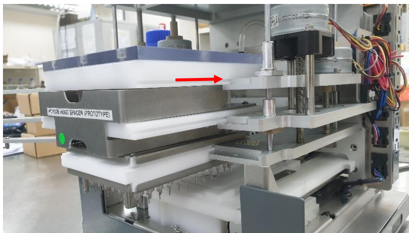
Figure 3-9: Align Fluidic Head to Machine (step 3)
