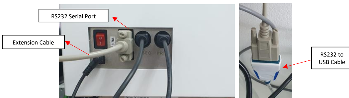
Figure 3-16: RS232 Serial Port Connection to HT2100 (left) and Computer/Laptop 7 (right).
