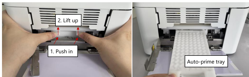
Figure 4.3: Disengage the Auto-prime tray from the spill tray (left). Slide the Auto-prime Tray out of the washer (right).
