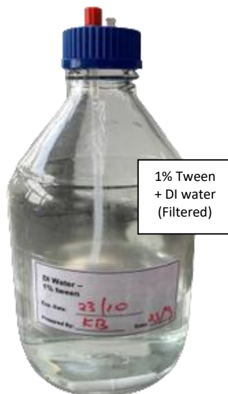
Figure 3-14: Buffer inlet bottle cap connected to 2L bottle containing wash buffer of choice.
