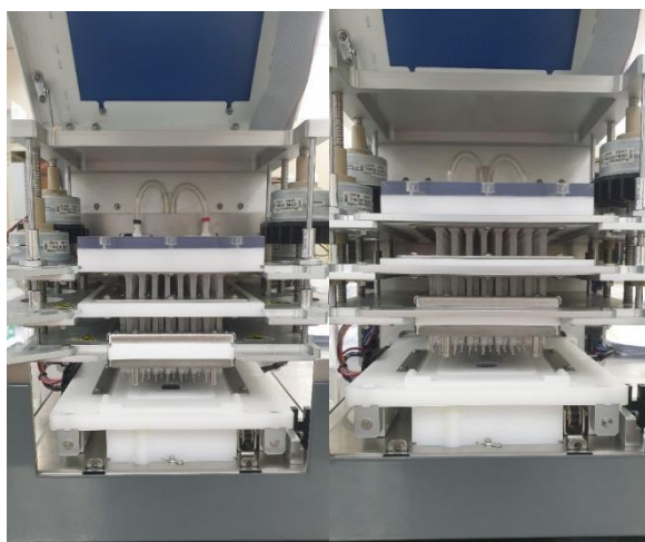
Figure 3.11: Align Fluidic Head to Machine (step 5)
