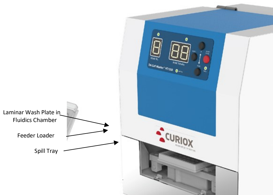
Figure 2-2: Lateral (right side) view of the Laminar Wash HT1000 with main components labeled.
