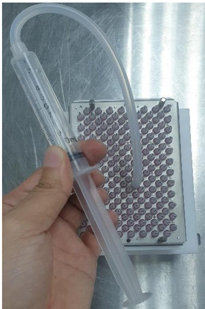
Figure 5-4: Manual syringe resetting of valve membrane
