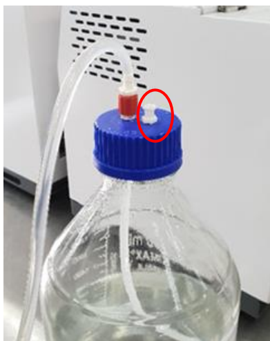
Figure 5-3: Release port on bottle cap
