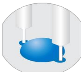
2 nozzles per droplet on Laminar Wash Plate.
