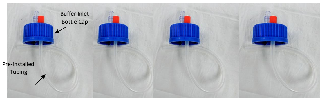
Figure 3-13: Four sets of buffer inlet bottle caps with pre-installed tubing
