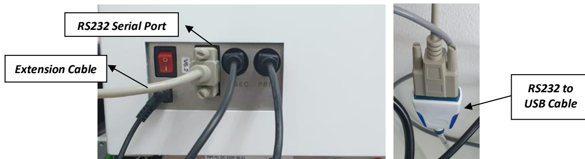
Figure 3-16: RS232 Serial Port Connection to Computer/Laptop 7
