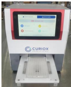
Figure 3-18: Insert priming plate into machine (in [Service Mode])
