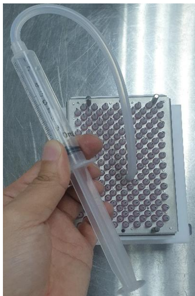
Figure 5-4: Manual syringe resetting of valve membrane
