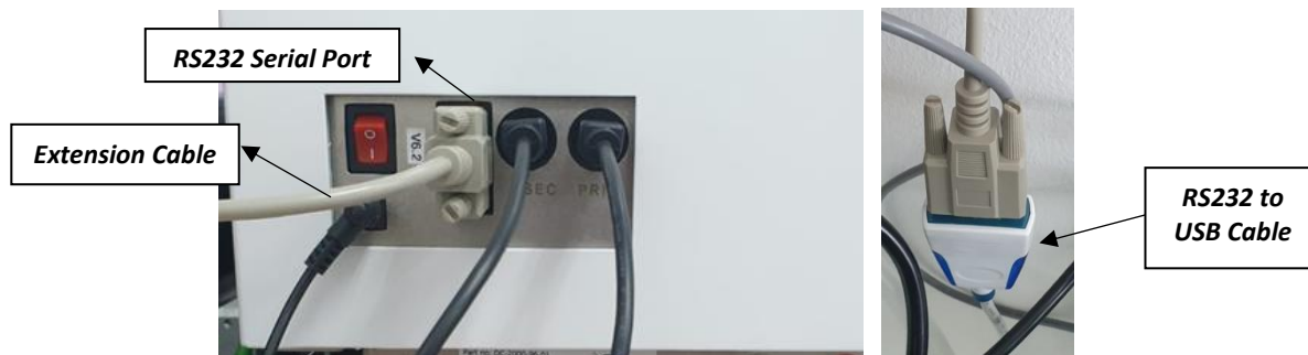
Figure 3-16: RS232 Serial Port Connection to Computer/Laptop 7
