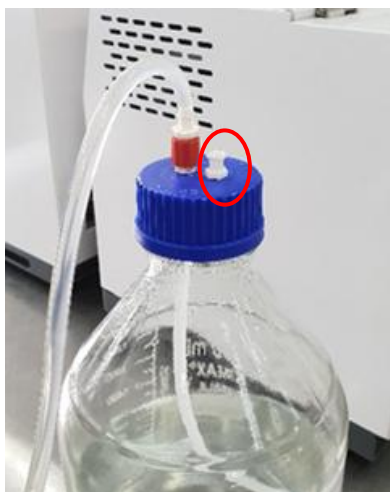
Figure 5-3: Release port on bottle cap
