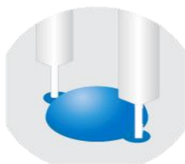
2 nozzles per droplet on Laminar Wash Plate.
