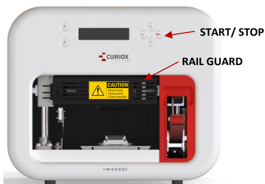
Figure 1-3: Stop Button and Rail Guard
