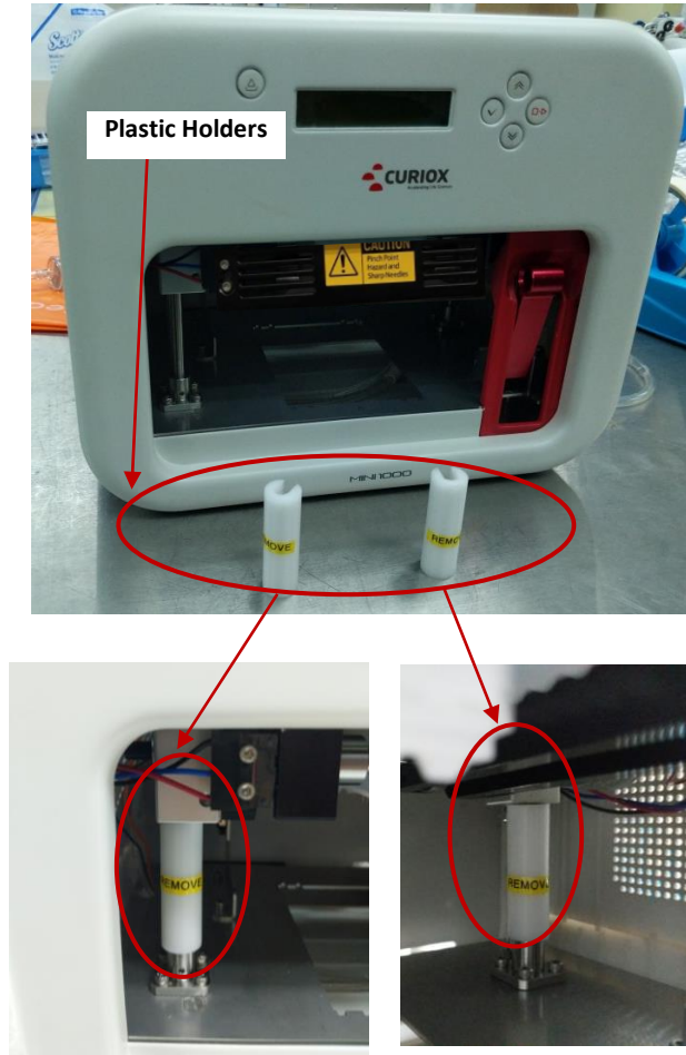
Figure 3-2: Unlocking machine pillar
